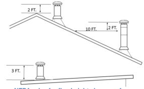
NFPA rules for flue height above roof
