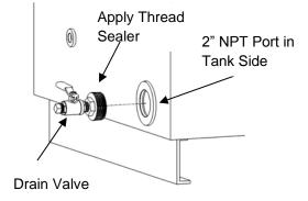
Drain valve installation.
