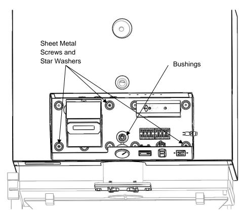
**Bushing Install and Cabinet Alignment**
