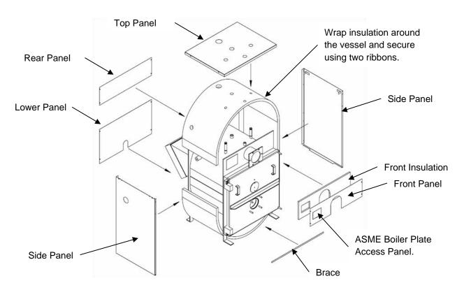
Assembling Insulation and Panels (EL-200B shown)
