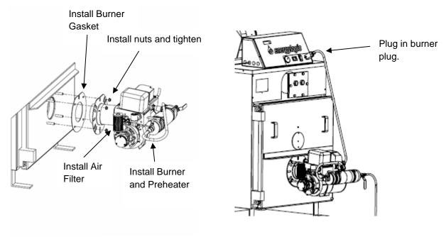
Installation of Burner on EL-200B.
