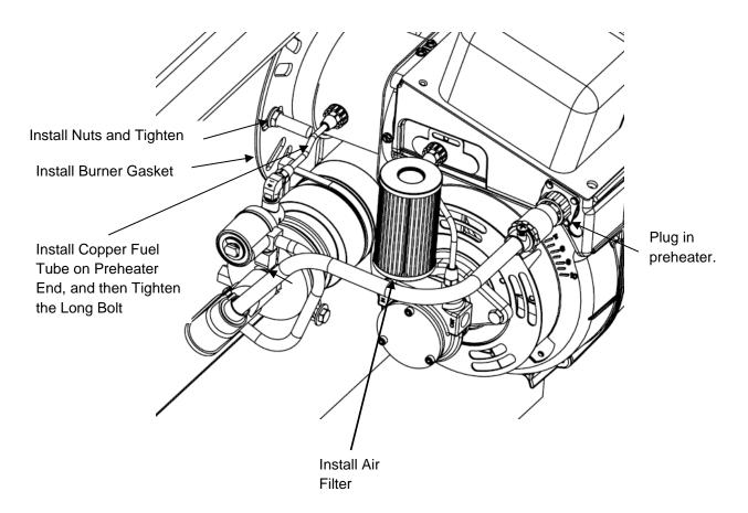
Installation of Burner on EL-375B and EL-500B.
