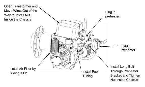
**EL-200B Preheater Assembly (to burner).**
