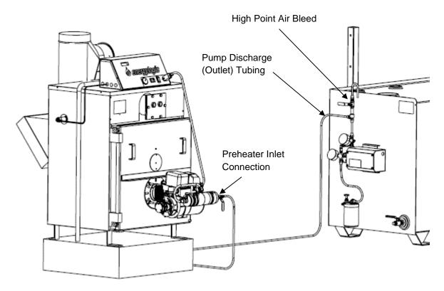
**Routing of Discharge Fuel Tubing - Tank Mount**
