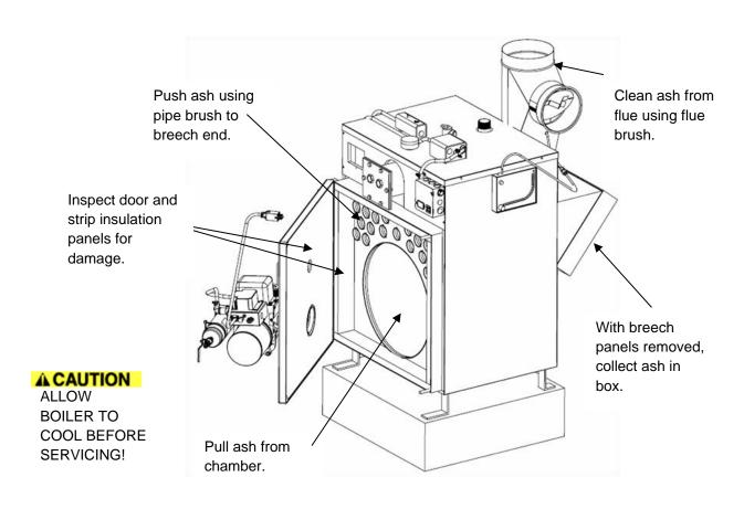
**Cleaning Heat Exchanger and Flue**
