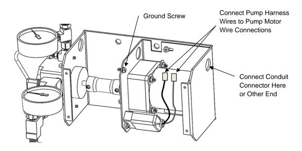
Wire Connections to the Metering Pump.
