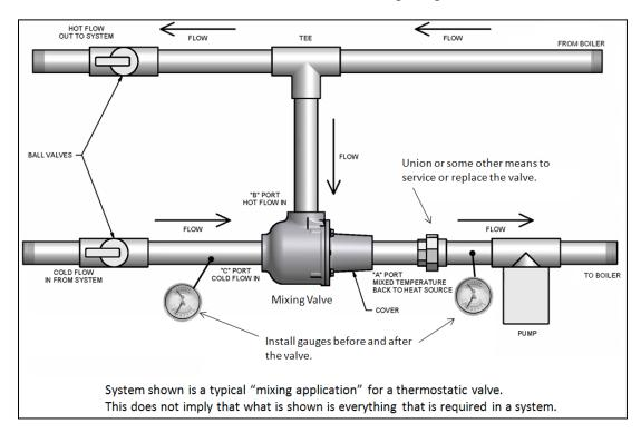
**Boiler Mixing Valve Arrangement**
