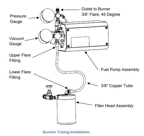
4. Tighten both flare nuts. Use a backup wrench - do not over-tighten.
