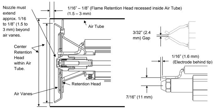
Settings for Retention Head & Electrodes - "Double Bend" Electrodes
