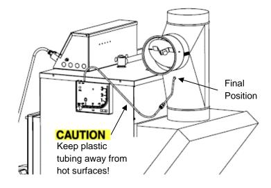
**Draft Gauge Probe Installation**
