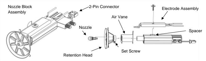
**Disassemble Nozzle Block**
